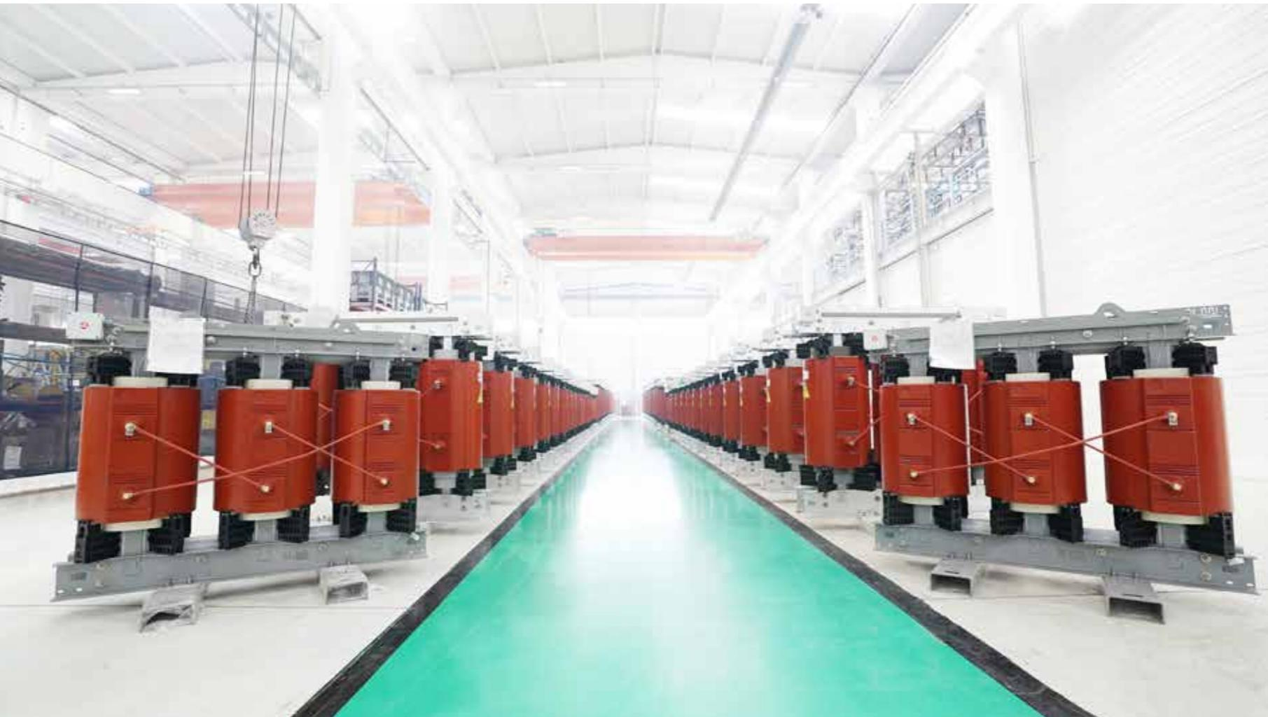
ASTOR Inc. manufactures natural air cooled (AN) or fan cooled (AF), cast resin dry type transformers up to 36 kV voltage and 25 MVA power capacity.
